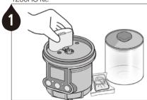
Remove the oil reservoir and check that the battery is properly installed.
